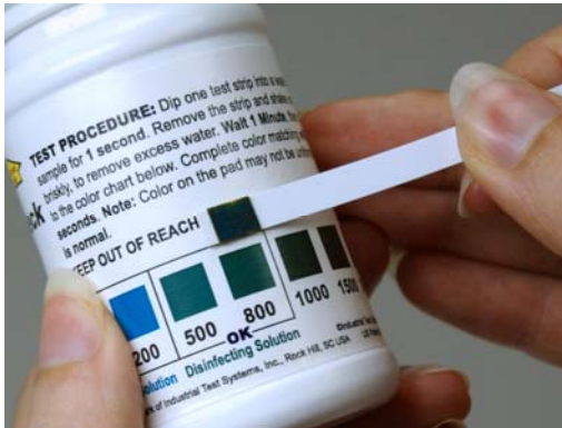
Testing disinfecting solution with Free Chlorine Ultra High II test strips 480124.
